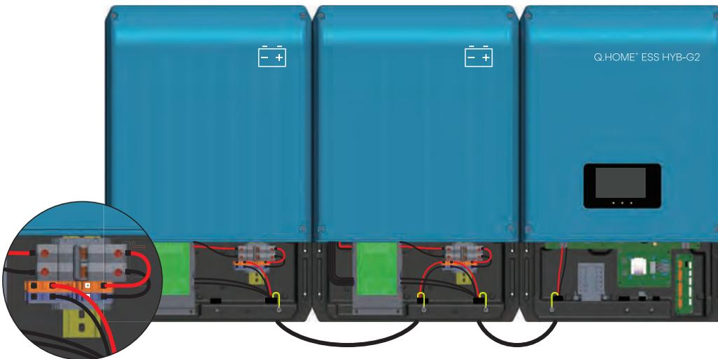
[ Figure 5-8 : Battery Pack and INVERTER Connection ]
