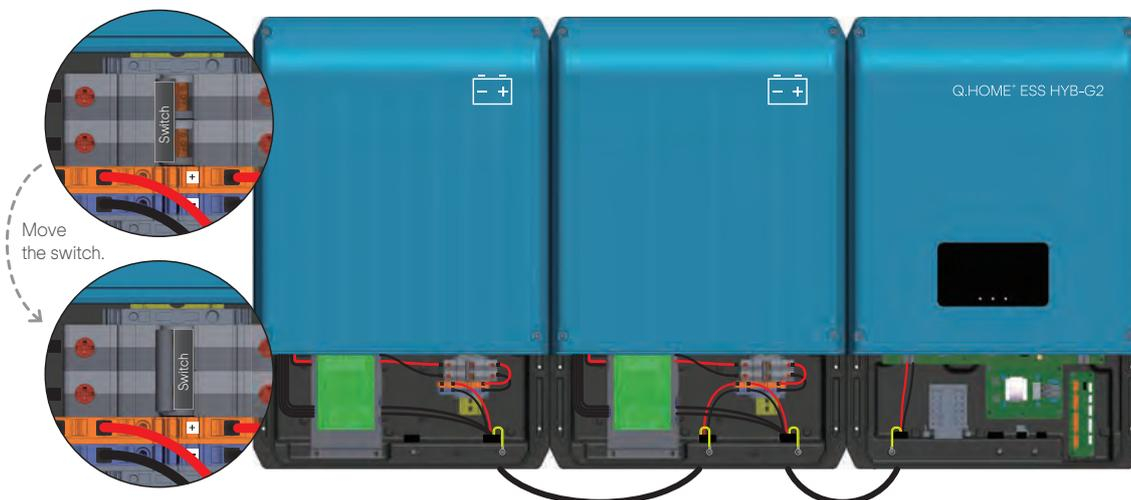
[ Figure 5-18 : Battery Pack Switch ]
